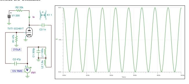
L1 and L2 are series connected coupled inductors (K=1).
