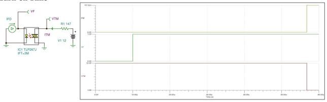
The turn-on time delay depends on the LED trigger current.
