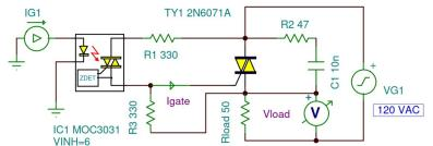
With typical inhibit voltage of 6 V, a TRIAC gate could require 8 mA at -20 °C (Rmax=6 V/8 mA = 750 Ω). By using 330 Ω for the gate resistor (R1), a current of at least 15 mA is supplied with only 5 V, but limited to 60 mA
