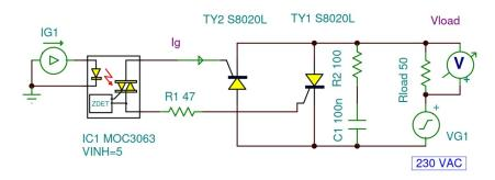
Zero voltage crossing turnon opto-drivers are designed to limit turn-on voltage to less than 20 V. Since the voltage is limited to 20 V or less, the series gate resistor that limits the gate drive current has to be much lower with a zero crossing opto-driver. With typical inhibit voltage
