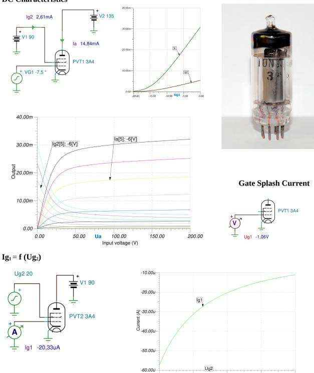
This model is valid for the following tubes (within max. ratings): DL93, 2P3, CV2390, CV807
