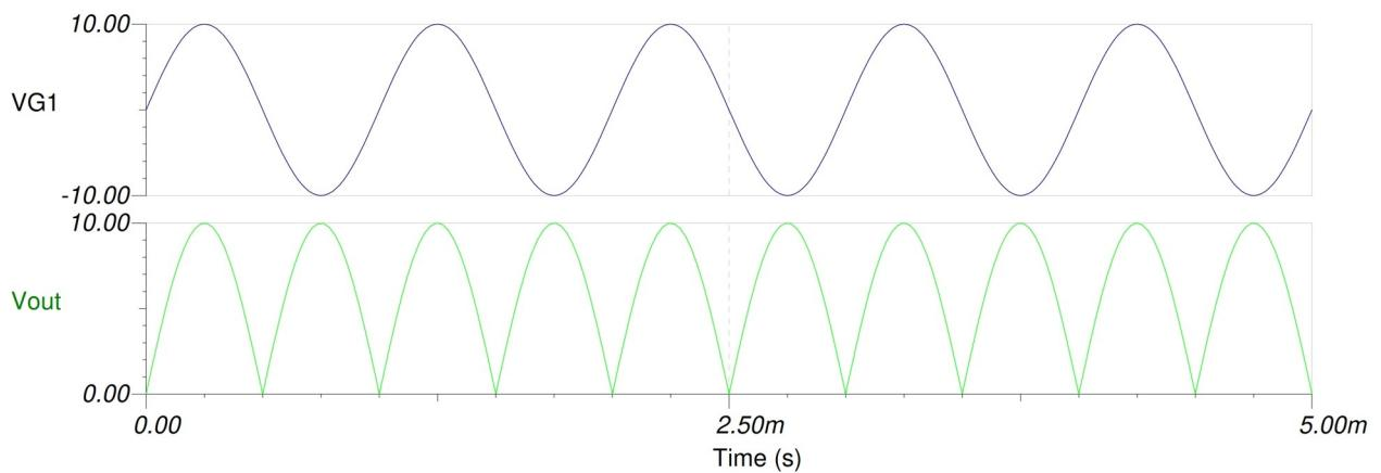
The precision rectifier circuit is convenient in that it only requires two op amps and that all resistors are the same value. This circuit consists of two parts: an inverting half-wave rectifier and a weighted summing amplifier.
