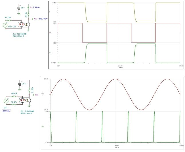
Typical values are for information only and are not part of the testing requirements. TLP292 is designed for applications requiring detection or monitoring of AC signals.
