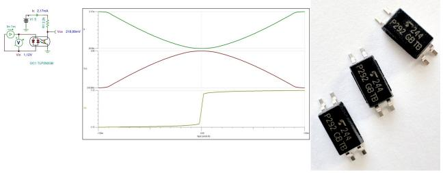
TLP292 is a low AC input type photocoupler that consists of phototransistor optically coupled to two antiparallel infrared LEDs in a SO4 package.
