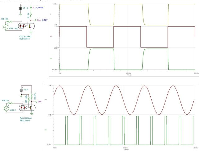
Typical values are for information only and are not part of the testing requirements. H11AA1 is designed for applications requiring detection or monitoring of AC signals.
