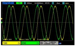
The quadrature oscillator is another type of phase-shift oscillator, but the three RC sections are configured so that each section contributes 90° of phase shift. The outputs are labeled sine and cosine (quadrature) because there is a 90° phase shift between op amp outputs.
