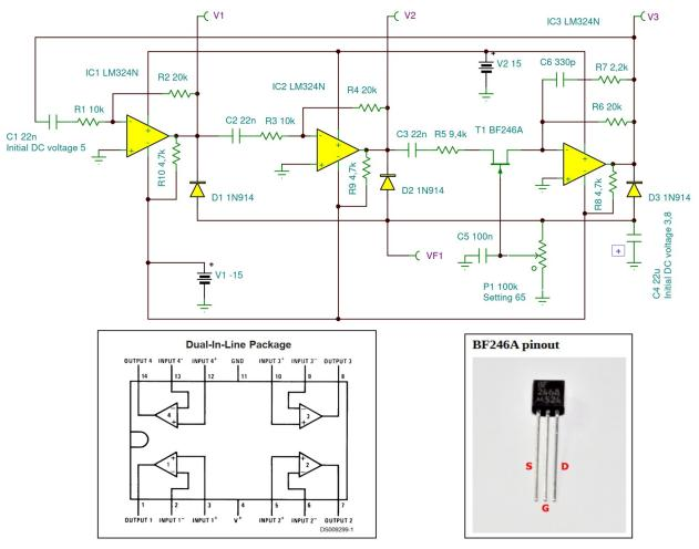
For ac applications, where the load is capacitively coupled to the output of the amplifier, a resistor should be used, from the output of the amplifier to ground (V-) to increase the class A bias current and prevent crossover distortion (R8, R9, R10).
