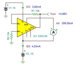
The <u>CA3140</u> Series circuits employ a broad band output stage that can sink loads to the negative supply to complement the capability of the PMOS input stage when operating near the negative rail. When the CA3140 is operating such that output Terminal 6 (OUT) is sinking current to the V- bus, transistor Q16 is the current sinking element. This sink current flows regardless of load; any excess current is internally supplied by the emitter-follower Q18.
