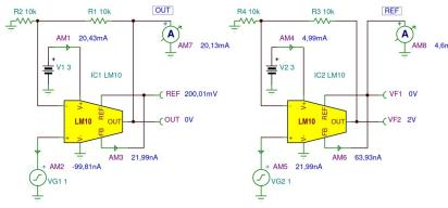
The input common-mode voltage range of the LM10 extends from the negative rail to 0.85 V less than the positive rail.
