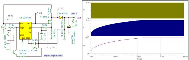
With current mode control, slope compensation is required to stabilize the overall loop with duty cycles exceeding 50%.
