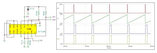
Either amplifier provided on the TL494 can be used for current limiting. Application of either amplifier is limited primarily to load-current control. The architecture defines that these amplifiers be used for *dc control applications*. Both amplifiers have a broad common-mode voltage range that allows direct current sensing at the output voltage rails. The internal architecture of the TL494 does not accommodate direct pulse-current limiting.
