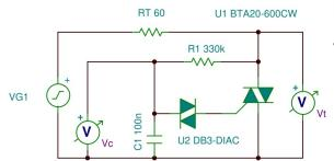
The R1 is used to control the applied voltage in both the half cycles .
